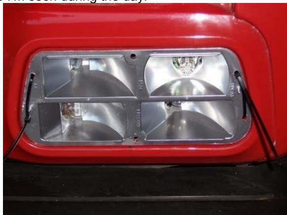
Repainted housing in body for trial fit – not my high-tech retaining clamps – I go through quite a few of those ties rebuilding things.
