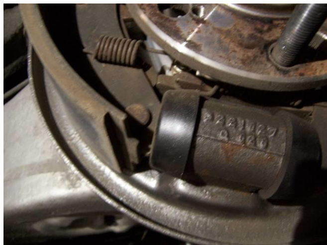
Behind that leading shoe on the driver's side lies the self adjuster that can give you conniptions - patience is the key
