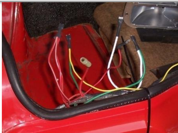
Wiring for the dual filament sockets
