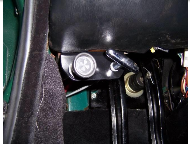
New bracket under the dash where the old bracket was, cables installed
