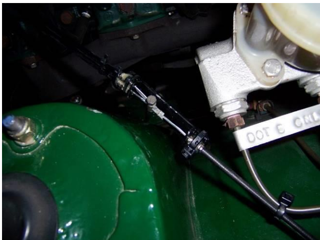
Inside cables soldered, barrel-clamped and in place
