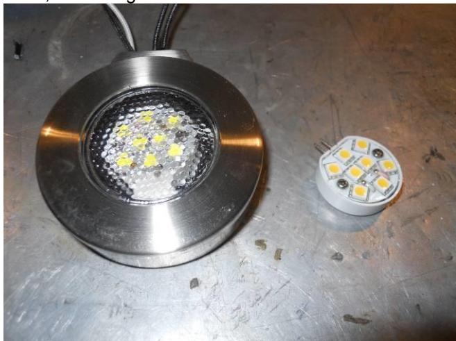
RV LED Fixture to the left, the LED bulb to the right
