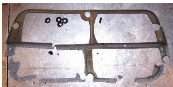
Old Tail Light Lens Gasket. Old gasket that has fallen apart. Bad gasket, bad!
