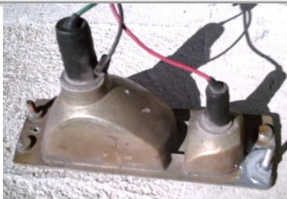
New stud epoxied on the old front turn signal housing – new stud to the right
