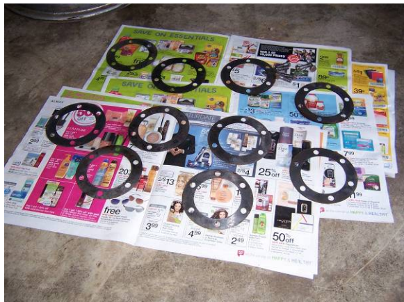
Shims left over after getting the hubs back on – don't know why all these are here since with about "0.02" on each side the play is in the recommended range.
