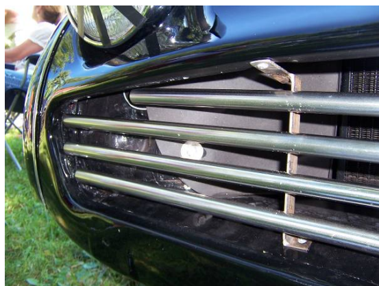
Stainless Tube Grill – a guy in Dayton that does TR3 interiors says he can make one for me - cool.
