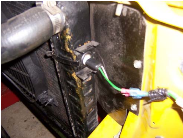
New-Old Fan Switch in place
