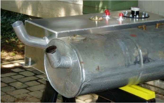
new tank after filler neck installed
