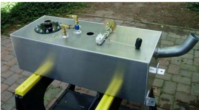
Tank with fittings and sending unit. The racing fuller cap isn't used.
