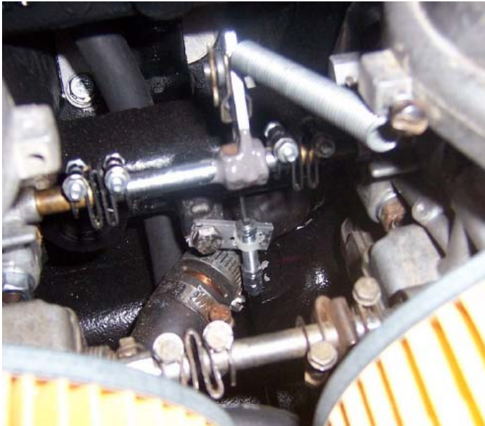
Up-Close and personal with the carb linkage. JB Weld is great stuff!
