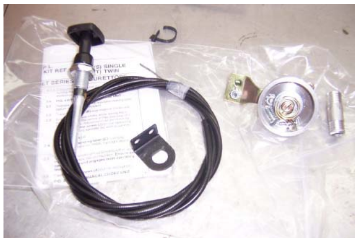
Moss Choke Conversion Kit – Stuff on the left is needed
