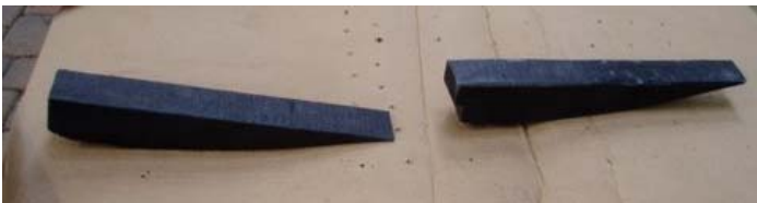
spacer to go under new tank, contoured to match inside body shape
