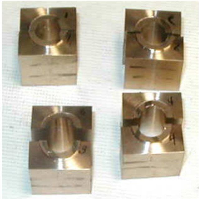
Then a trip to the lathe where the ends are surfaced and inside bored.
