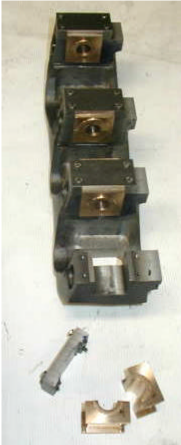
Another view of crankcase with bearings. That's the crankshaft sans the cranks through the bearings.
