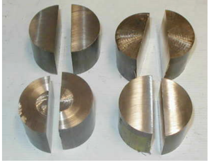
Then a trip to the mill where the bronze meets a fly cutter
