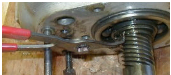
The next step is to remove the circlip on the main shaft to the rear of the center bearing using circlip pliers as shown in next photo.
