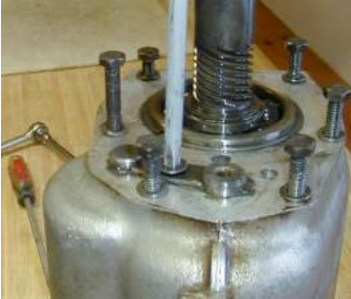
After the retaining plate is removed the countershaft can be removed to the rear by placing a long rod against the front of the countershaft and tapping gently with a small hammer as shown in the next two photos.
