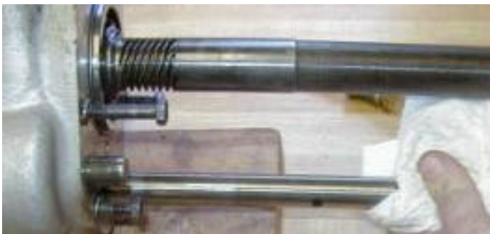
Once the countershaft is removed the countershaft gears drop to the bottom of the gearbox permitting the input shaft and main shaft to be removed.
