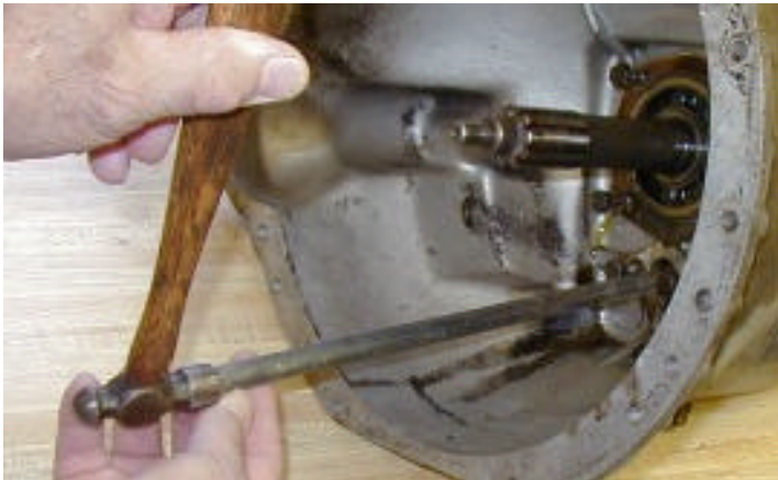
After the retaining plate is removed the countershaft can be removed to the rear by placing a long rod against the front of the countershaft and tapping gently with a small hammer as shown in the next two photos.
