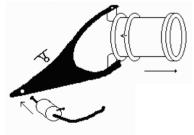
Possible improper fit due to over-extension of the clutch arm during gearbox installation
