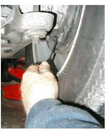
Adjusting the Handbrake Cables: Recall that there is a compensator between the hand brake lever and cables to balance the force on the two cables. Because of this, care should be taken to adjust the two cables to the same length. Otherwise, the compensator might reach the extreme of the balancing capability and apply more force to one wheel. I adjust the brakes as described above before adjusting the cables.
