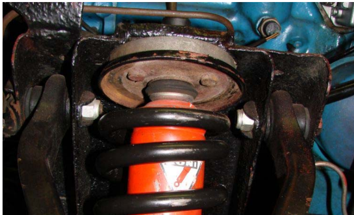
Figure 5 Big gaps at top of the shocks
