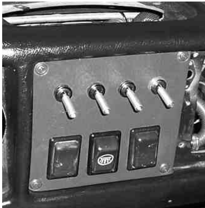
New Switch Panel - Who Needs Stinking Vents? Notice I Kept The Original Window & Light Switches
