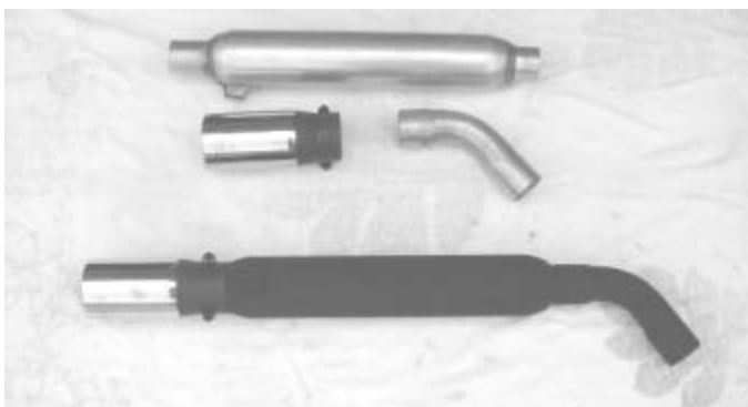
Top: All the Parts. Bottom: Completed Side Exhaust
