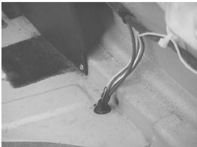
Hole In Trunk Where Wires Go Through
