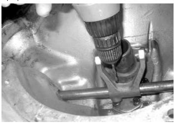
Drilling hole in clutch fork
