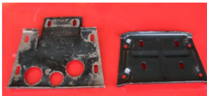
Figure 3 Cracked bracket on the left
