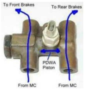
The PDWA is equipped with an electrical switch that operates if the piston moves off center. The end of the switch and piston are shown in the photo below. The switch plunger normally rides in the narrow part on the center of the piston. If the piston moves off center, a larger diameter part of the piston comes under the switch and pushes the plunger into the switch, operating the switch in the process. The operated switch will then turn on the BRAKE warning lamp on the dash.
