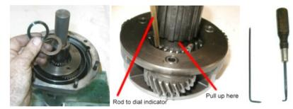
The left photo below shows the actual setup. A fairly large steel bar was used to secure the indicator magnetic base and provide stability. The right photo shows a young LBC mechanic wanabe at work.
