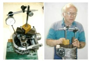
**No End Float!** When the end float was measured with the dial indicator there was none. That was the same result I got using the extra washer method --- but the problems mentioned earlier caused variations of about .010 inch so I didn't know for sure. A problem was suspected because the thrust washer had a grove worn in it. Also, remember that the thrust washer between the sun gear and planet carrier had been destroyed.
