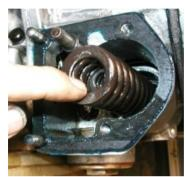
**Installing the Pump Non-Return Valve:** The pump non-return valve is identical the the operating valve installed earlier except there is no long spindle. The parts were lubricated and then the ball, plunger and spring were dropped into the hole. The plug with copper washer was then screwed in and tightened.
