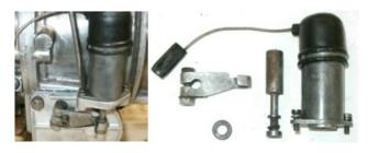
The cover that retains the humongous accumulator spring was removed next. It is secured by two bolts to the rear and two nuts on studs toward the front and must be removed properly so that it is not bent or distorted. Caution, the operating valve must be operated and released a half dozen
