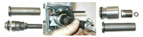
**Removing Non-Return Valve:** The pump non-return valve is located beside the accumulator cylinder as shown in the left photo below. After the plug was removed the spring, plunger washer, and ball were removed, cleaned, inspected and stored (right photo).
