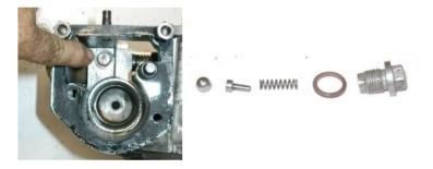
**Removing Pump:** The drain plug and screen filter must be removed to expose the pump. The photos below were taken after the gearbox had been cleaned up. Much of the oil evaporated from the heat generated when the bearing failed. The outside of the screen was covered by black goo mixed with metal parts. (The later models use a larger plug and the screen is retained by the plug rather than the screw as shown in photos below.)
