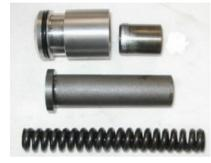
It is possible to replace the earlier accumulator with the later accumulator (the housing, piston, spacing tune and spring are all required). The Victoria British Catalog suggests this option if replacement springs, piston or rings are required for the early accumulator.
